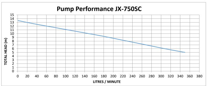
**NOTE:** The above Performance graph is measured at pump outlet and based on factory test conditions. Actual performance onsite may differ due to piping and fixture sizing and layout
